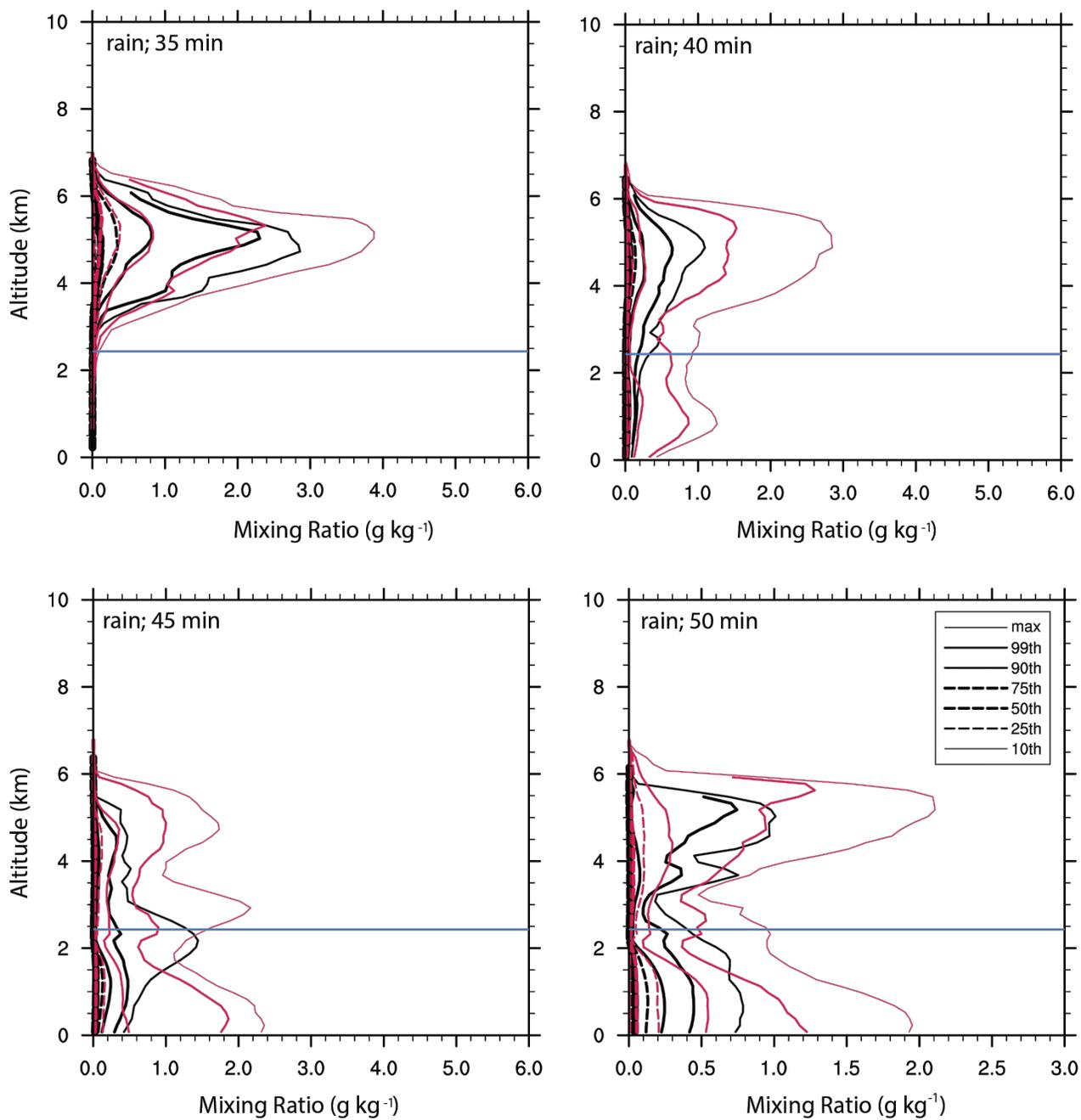
Fig. 1. Contoured frequency by altitude diagrams (CFADs) of rain mass for the 2 Aug control simulation (black) and another 2 Aug simulation with half the vertical wind shear (red). Reducing the vertical wind shear, all else being the same as the control run, greatly increased the surface rainfall. The height of the environmental 0°C isotherm is shown by a blue horizontal line. Adapted from Lasher-Trapp et al. (2018).
